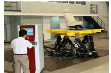
Figure 6: Shaking table for frequency response experiment
